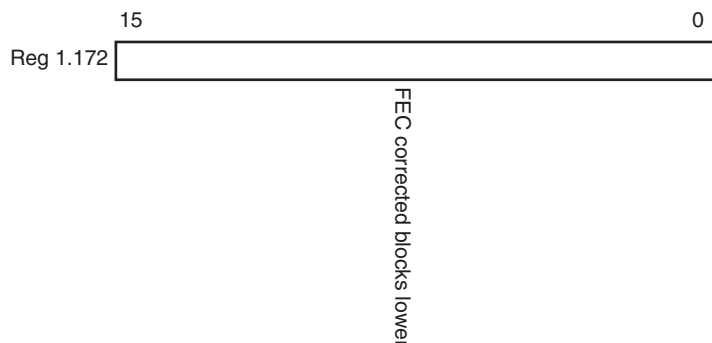
Figure 6-26: 10GBASE-R FEC Corrected Blocks (Lower) Register
