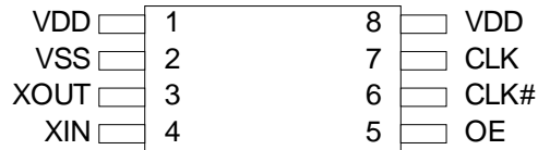
Figure 1. 8-pin TSSOP pinout
