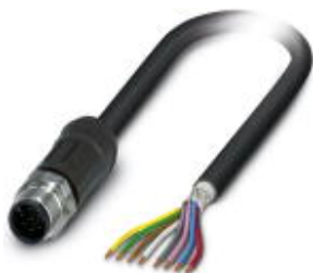
Sensor/Actuator cable, 8-position, PE-X/PE-X halogen-free, black-gray RAL 7021, shielded, Plug straight M12, A-coded, on free cable end, Cable length: 5 m, for outdoor applications, with high-grade steel knurl
