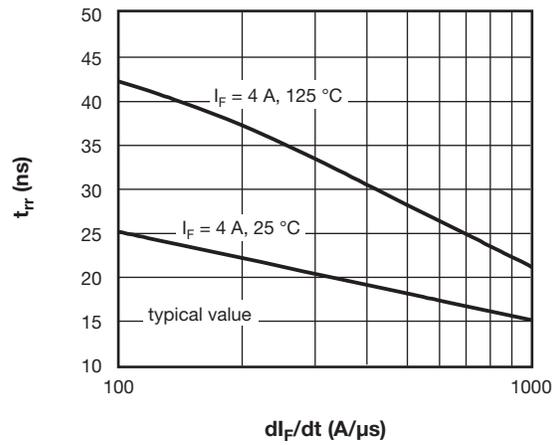
Fig. 6 - Typical Reverse Recovery vs.  $dI_F/dt$
