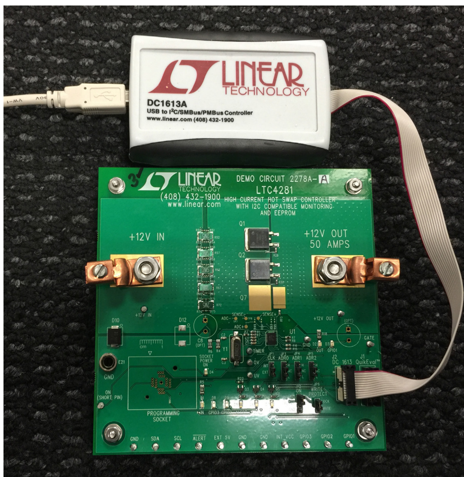
Figure 2. DC2278A-A Demo Board Connected to DC1613 I 2 C-to-USB Converter
