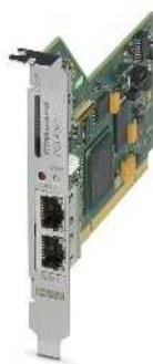
Router with firewall and VPN for PCI
