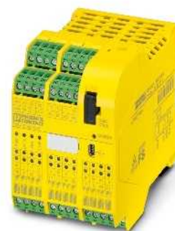
Configurable safety module, can be extended
