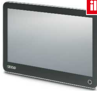
Fully enclosed IP65 IPC with 47 cm (18.5") display
