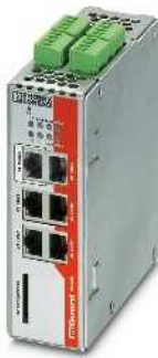
Router with simplified 2-click firewall, VPN, and integrated switch
