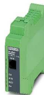
Modem for dial-up operation with USB connection
