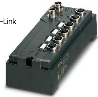
4 IO-Link ports and 4 digital inputs
