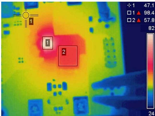
Figure 21: Thermal Image at V_{IN} = 12V , I_{OUT} = 12A (IR3476: 98^\circ C , Inductor: 58^\circ C , PCB: 47^\circ C )
