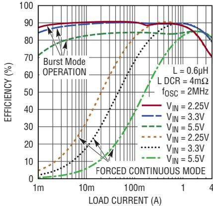
**4A Buck Efficiency vs  $I_{LOAD}$ ,  $V_{OUT} = 1.8\text{V}$**
