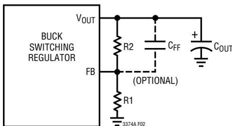
Figure 2. Feedback Components
