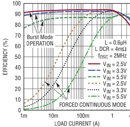
**4A Buck Efficiency vs  $I_{LOAD}$ ,  $V_{OUT} = 2.5\text{V}$**
