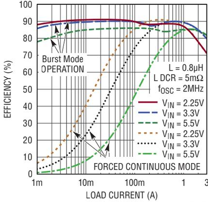
**3A Buck Efficiency vs  $I_{LOAD}$ ,  $V_{OUT} = 1.8\text{V}$**
