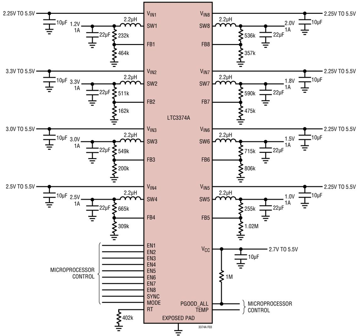
Figure 3. Detailed Front Page Application (All 1A Outputs)
