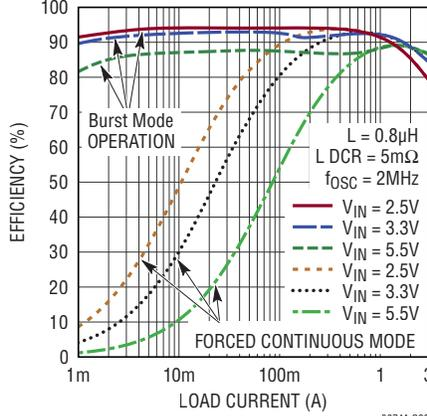
**3A Buck Efficiency vs  $I_{LOAD}$ ,  $V_{OUT} = 2.5\text{V}$**
