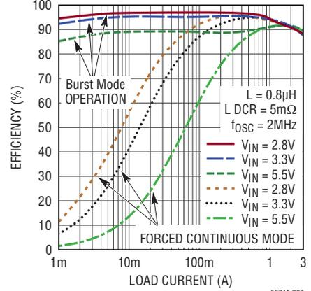
**4A Buck Efficiency vs  $I_{LOAD}$ ,  $V_{OUT} = 1.2\text{V}$**
