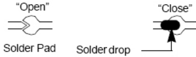
Figure 2-6. Solder Strap Definition
