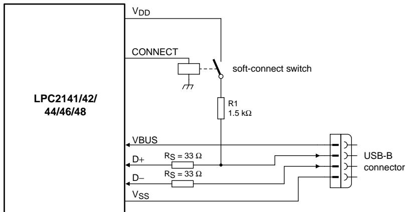
Fig 10. LPC2141/42/44/46/48 USB interface using the CONNECT function on pin 17
