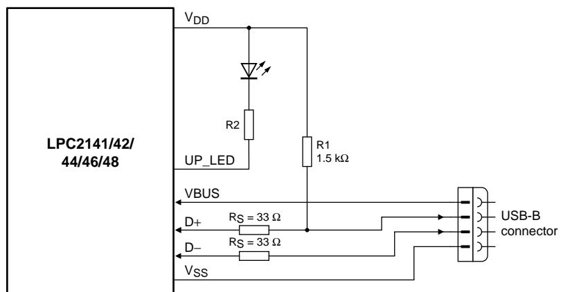
Fig 11. LPC2141/42/44/46/48 USB interface using the UP\_LED function on pin 17
