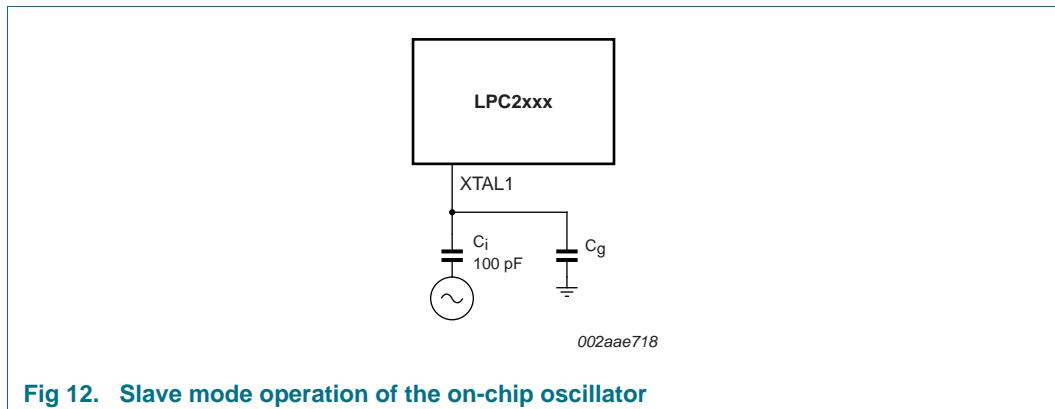
**Fig 12.** Slave mode operation of the on-chip oscillator
