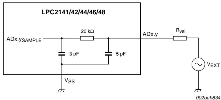
Fig 9. Suggested ADC interface - LPC2141/42/44/46/48 ADx.y pin
