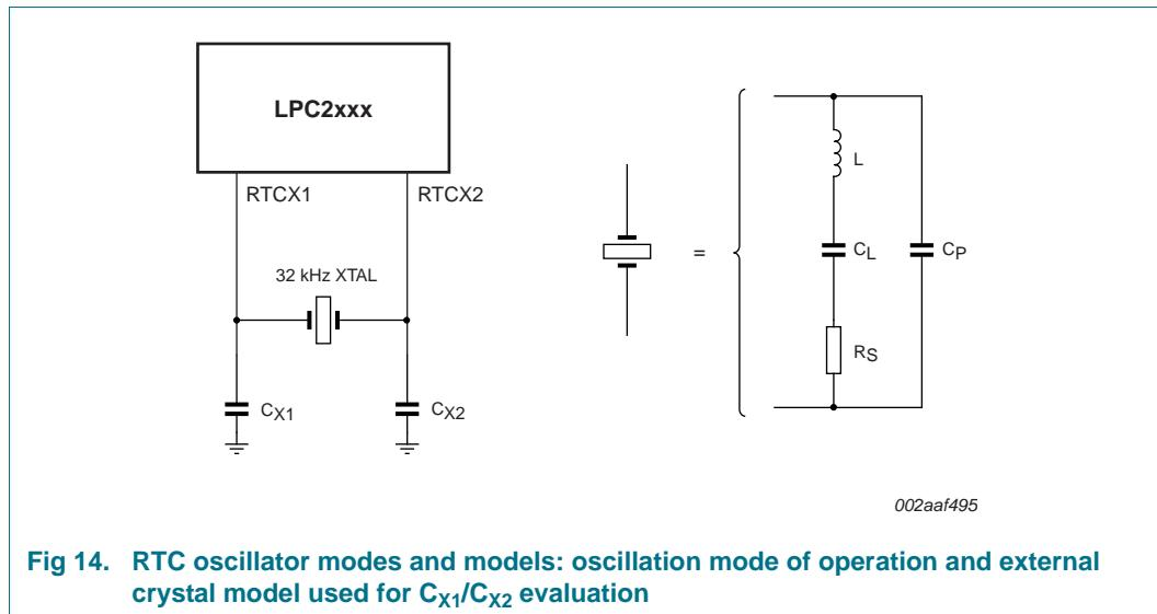
**Fig 14.** RTC oscillator modes and models: oscillation mode of operation and external crystal model used for  $C_{X1}/C_{X2}$  evaluation
