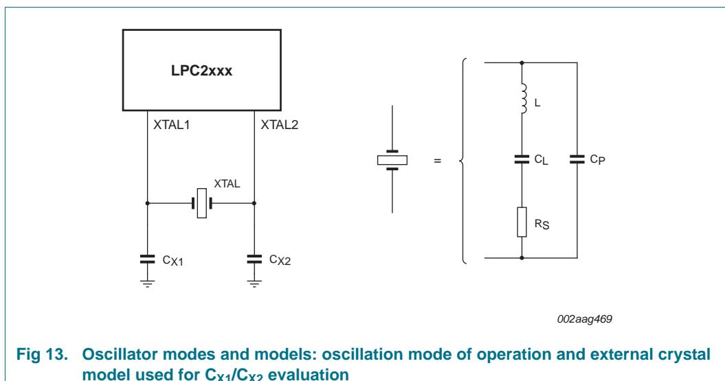
**Fig 13.** Oscillator modes and models: oscillation mode of operation and external crystal model used for  $C_{X1}/C_{X2}$  evaluation**Table 10.** Recommended values for  $C_{X1}/C_{X2}$  in oscillation mode (crystal and external components parameters): low frequency mode
