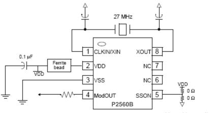
Use either pull-up or pull-down resistors with 0  $\Omega_{\rm \cdot}$
