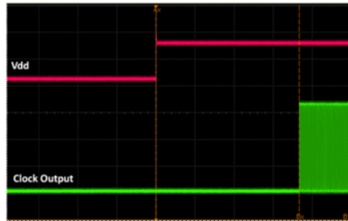
Figure 17. Startup Waveform vs. Vdd
