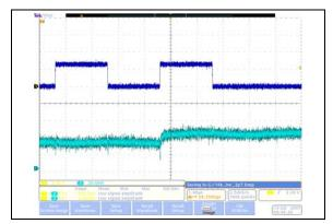
**FIGURE 2-29:** 10  $k\Omega$  – Low-Voltage Increment Wiper Settling Time ( $V_{DD}$  = 2.7V) (1  $\mu$ s/Div).
