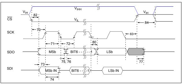
FIGURE 1-2: SPI Timing Waveform (Mode = 00).
