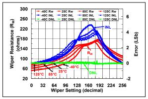
**FIGURE 2-9:** 5  $k\Omega$  Rheo Mode –  $R_W$  ( $\Omega$ ), INL (LSb), DNL (LSb) vs. Wiper Setting and Ambient Temperature ( $V_{DD} = 3.0V$ ).
