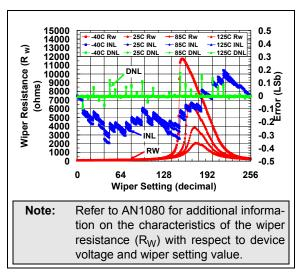
**FIGURE 2-32:** 50  $k\Omega$  Pot Mode –  $R_W$  ( $\Omega$ ), INL (LSb), DNL (LSb) vs. Wiper Setting and Ambient Temperature ( $V_{DD}$  = 1.8V).
