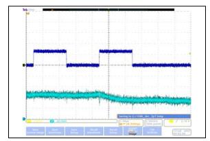
**FIGURE 2-51:** 100 kΩ – Low-Voltage Decrement Wiper Settling Time ( $V_{DD}$  = 2.7V) (1 μs/Div).
