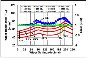
**FIGURE 2-21:** 10 kΩ Rheo Mode –  $R_W$  (Ω), INL (LSb), DNL (LSb) vs. Wiper Setting and Ambient Temperature ( $V_{DD}$  = 5.5V).
