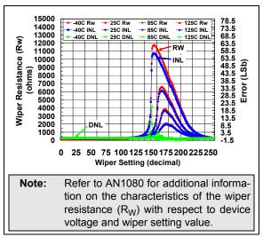
**FIGURE 2-35:** 50 k $\Omega$  Rheo Mode –  $R_W(\Omega)$ , INL (LSb), DNL (LSb) vs. Wiper Setting and Ambient Temperature ( $V_{DD} = 1.8V$ ).
