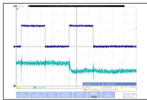
**FIGURE 2-26:** 10 k $\Omega$  – Low-Voltage Decrement Wiper Settling Time ( $V_{DD} = 5.5V$ ) (1  $\mu$ s/Div).
