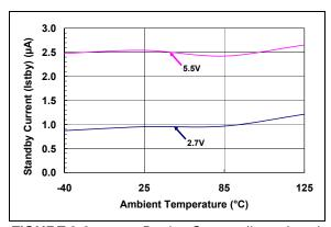
**FIGURE 2-2:** Device Current ( $I_{SHDN}$ ) and  $V_{DD}$ .  $(\overline{CS} = V_{DD})$  vs. Ambient Temperature.
