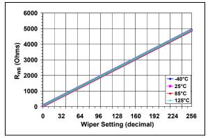
**FIGURE 2-12:**  $5 k\Omega - R_{WB} (\Omega)$  vs. Wiper Setting and Ambient Temperature.
