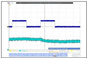
**FIGURE 2-39:** 50 kΩ – Low-Voltage Decrement Wiper Settling Time ( $V_{DD} = 2.7V$ ) (1 μs/Div).
