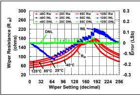
**FIGURE 2-31:** 50 kΩ Pot Mode –  $R_W$  (Ω), INL (LSb), DNL (LSb) vs. Wiper Setting and Ambient Temperature ( $V_{DD}$  = 3.0V).
