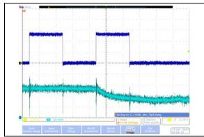
**FIGURE 2-50:** 100 k $\Omega$  – Low-Voltage Decrement Wiper Settling Time ( $V_{DD}$  = 5.5V) (1  $\mu$ s/Div).
