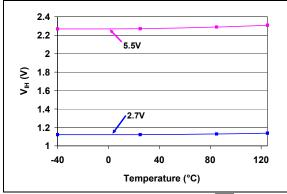
**FIGURE 2-58:**  $V_{IH}$  (SDI, SCK,  $\overline{CS}$ , and  $\overline{SHDN}$ ) vs.  $V_{DD}$  and  $\overline{Temperature}$ .
