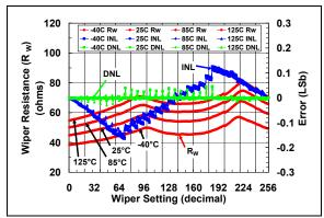
**FIGURE 2-30:** 50 k $\Omega$  Pot Mode –  $R_W$  ( $\Omega$ ), INL (LSb), DNL (LSb) vs. Wiper Setting and Ambient Temperature ( $V_{DD} = 5.5V$ ).
