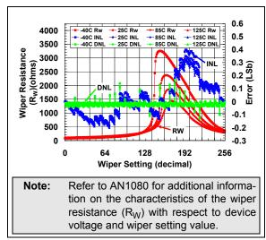
**FIGURE 2-20:** 10  $k\Omega$  Pot Mode –  $R_W$  ( $\Omega$ ), INL (LSb), DNL (LSb) vs. Wiper Setting and Ambient Temperature ( $V_{DD} = 1.8V$ ).
