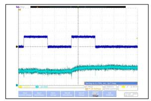
**FIGURE 2-41:** 50 k $\Omega$  – Low-Voltage Increment Wiper Settling Time ( $V_{DD}$  = 2.7V) (1  $\mu$ s/Div).
