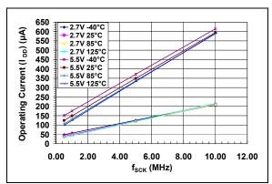
**FIGURE 2-1:** Device Current ( $I_{DD}$ ) vs. SPI Frequency ( $f_{SCK}$ ) and Ambient Temperature ( $V_{DD} = 2.7V$  and 5.5V).
