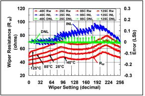
**FIGURE 2-45:** 100 kΩ Rheo Mode –  $R_W$  (Ω), INL (LSb), DNL (LSb) vs. Wiper Setting and Ambient Temperature ( $V_{DD}$  = 5.5V).
