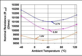
**FIGURE 2-24:** 10  $k\Omega$  – Nominal Resistance  $(\Omega)$  vs. Ambient Temperature and  $V_{DD}$ .
