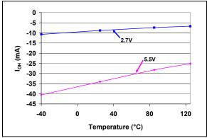
**FIGURE 2-60:**  $I_{OH}$  (SDO) vs.  $V_{DD}$  and Temperature.
