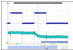
**FIGURE 2-38:** 50 kΩ – Low-Voltage Decrement Wiper Settling Time ( $V_{DD} = 5.5V$ ) (1 μs/Div).
