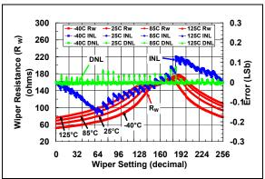
**FIGURE 2-19:** 10 kΩ Pot Mode –  $R_W$  (Ω), INL (LSb), DNL (LSb) vs. Wiper Setting and Ambient Temperature ( $V_{DD}$  = 3.0V).
