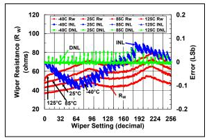
**FIGURE 2-42:** 100  $k\Omega$  Pot Mode –  $R_W$  ( $\Omega$ ), INL (LSb), DNL (LSb) vs. Wiper Setting and Ambient Temperature ( $V_{DD}$  = 5.5V).
