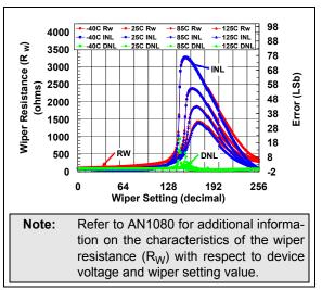
**FIGURE 2-23:** 10  $k\Omega$  Rheo Mode –  $R_W(\Omega)$ , INL (LSb), DNL (LSb) vs. Wiper Setting and Ambient Temperature ( $V_{DD} = 1.8V$ ).
