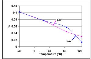
**FIGURE 2-56:** Resistor Network 0 to Resistor Network 1  $R_{AB}$  (50  $k\Omega$ ) Mismatch vs.  $V_{DD}$  and Temperature.
