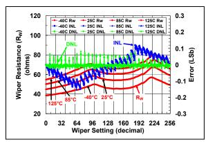
**FIGURE 2-5:**  $5 \text{ k}\Omega \text{ Pot Mode} - R_W (\Omega)$ , INL (LSb), DNL (LSb) vs. Wiper Setting and Ambient Temperature ( $V_{DD} = 5.5V$ ).
