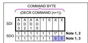
**Note 1:** Only functions when writing the volatile wiper registers (AD3:AD0) 0h and 1h.
