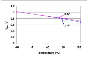
**FIGURE 2-62:** POR/BOR Trip point vs. V<sub>DD</sub> and Temperature.
