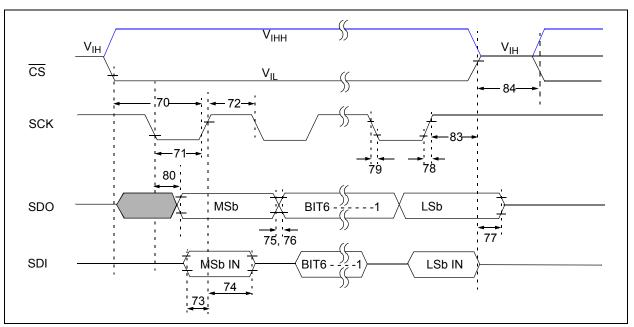
FIGURE 1-1: SPI Timing Waveform (Mode = 11).
