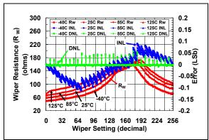
**FIGURE 2-43:** 100 k $\Omega$  Pot Mode –  $R_W$  ( $\Omega$ ), INL (LSb), DNL (LSb) vs. Wiper Setting and Ambient Temperature ( $V_{DD} = 3.0V$ ).
