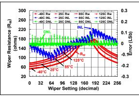
**FIGURE 2-6:** 5  $k\Omega$  Pot Mode –  $R_W$  ( $\Omega$ ), INL (LSb), DNL (LSb) vs. Wiper Setting and Ambient Temperature ( $V_{DD} = 3.0V$ ).
