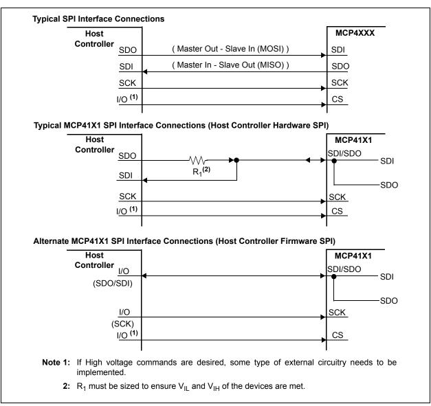
FIGURE 6-1: Typical SPI Interface Block Diagram.
