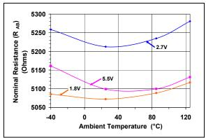
**FIGURE 2-11:** 5  $k\Omega$  – Nominal Resistance  $(\Omega)$  vs. Ambient Temperature and  $V_{DD}$ .
