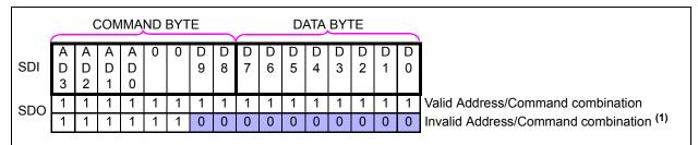
Note 1: If an Error Condition occurs (CMDERR = L), all following SDO bits will be low until the CMDERR condition is cleared (the CS pin is forced to the inactive state).
