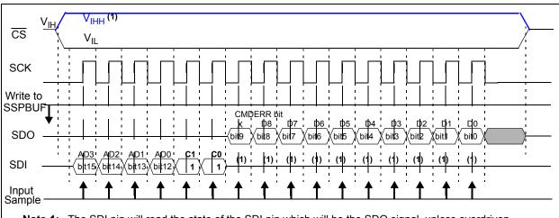
Note 1: The SDI pin will read the state of the SDI pin which will be the SDO signal, unless overdriven.
