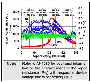
**FIGURE 2-7:** 5  $k\Omega$  Pot Mode –  $R_W$  ( $\Omega$ ), INL (LSb), DNL (LSb) vs. Wiper Setting and Ambient Temperature ( $V_{DD}$  = 1.8V).
