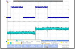
**FIGURE 2-16:**  $5 \text{ k}\Omega - \text{Low-Voltage}$ Increment Wiper Settling Time ( $V_{DD} = 5.5V$ ) (1  $\mu$ s/Div).
