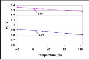
**FIGURE 2-59:**  $V_{IL}$  (SDI, SCK,  $\overline{CS}$ , and  $\overline{SHDN}$ ) vs.  $V_{DD}$  and Temperature.
