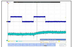
**FIGURE 2-53:** 100 k $\Omega$  – Power-Up Wiper Response Time (1 μs/Div).
