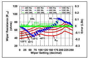
**FIGURE 2-18:** 10  $k\Omega$  Pot Mode –  $R_W$  ( $\Omega$ ), INL (LSb), DNL (LSb) vs. Wiper Setting and Ambient Temperature ( $V_{DD} = 5.5V$ ).
