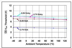
**FIGURE 2-4:**  $\overline{\text{CS}}$  High Input Entry/Exit Threshold vs. Ambient Temperature and V<sub>DD</sub>.
