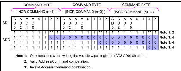
4: If an Error Condition occurs (CMDERR = L), all following SDO bits will be low until the CMDERR condition is cleared (the CS pin is forced to the inactive state).
