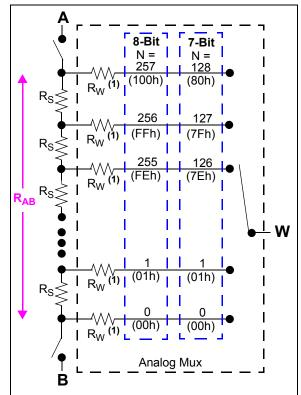
Note 1: The wiper resistance is dependent on several factors including, wiper code, device V<sub>DD</sub>, Terminal voltages (on A, B, and W), and temperature.
