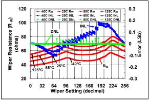
**FIGURE 2-33:** 50 k $\Omega$  Rheo Mode –  $R_W(\Omega)$ , INL (LSb), DNL (LSb) vs. Wiper Setting and Ambient Temperature ( $V_{DD} = 5.5V$ ).
