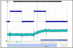
**FIGURE 2-52:** 100  $k\Omega$  – Low-Voltage Increment Wiper Settling Time ( $V_{DD}$  = 2.7V) (1  $\mu$ s/Div).
