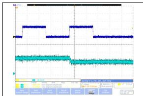
**FIGURE 2-14:**  $5 k\Omega$  – Low-Voltage Decrement Wiper Settling Time (V<sub>DD</sub> = 2.7V) (1 μs/Div).
