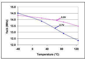
**FIGURE 2-63:** SCK Input Frequency vs. Voltage and Temperature.
