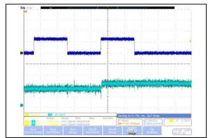
**FIGURE 2-17:**  $5 \, k\Omega - \text{Low-Voltage}$ Increment Wiper Settling Time ( $V_{DD} = 2.7V$ ) (1  $\mu$ s/Div).
