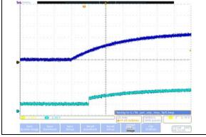
**FIGURE 2-15:**  $5 \, k\Omega$  – Power-Up Wiper Response Time (20 ms/Div).
