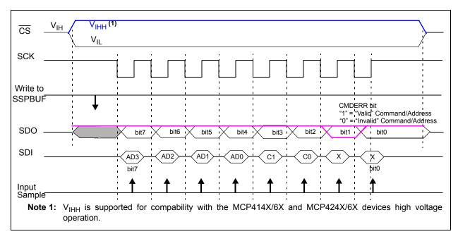
**FIGURE 6-7:** 8-Bit Commands (Increment, Decrement, Modify - SPI Waveform with PIC MCU (Mode 1,1).
