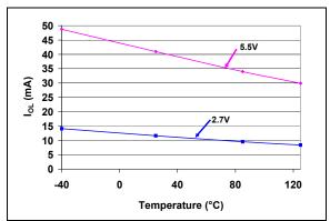
**FIGURE 2-61:**  $I_{OL}$  (SDO) vs.  $V_{DD}$  and Temperature.
