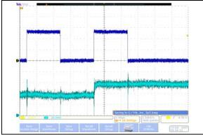
**FIGURE 2-28:** 10  $k\Omega$  – Low-Voltage Increment Wiper Settling Time ( $V_{DD} = 5.5V$ ) (1  $\mu$ s/Div).
