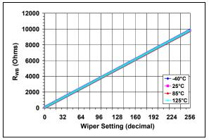
**FIGURE 2-25:** 10  $k\Omega$  –  $R_{WB}$  ( $\Omega$ ) vs. Wiper Setting and Ambient Temperature.
