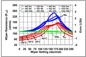
**FIGURE 2-22:** 10 k $\Omega$  Rheo Mode –  $R_W(\Omega)$ , INL (LSb), DNL (LSb) vs. Wiper Setting and Ambient Temperature ( $V_{DD} = 3.0V$ ).
