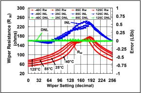
**FIGURE 2-34:** 50 k $\Omega$  Rheo Mode –  $R_W(\Omega)$ , INL (LSb), DNL (LSb) vs. Wiper Setting and Ambient Temperature ( $V_{DD} = 3.0V$ ).
