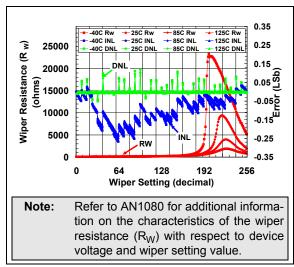
**FIGURE 2-44:** 100  $k\Omega$  Pot Mode –  $R_W$  ( $\Omega$ ), INL (LSb), DNL (LSb) vs. Wiper Setting and Ambient Temperature ( $V_{DD} = 1.8V$ ).
