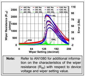
**FIGURE 2-10:** 5  $k\Omega$  Rheo Mode –  $R_W$  ( $\Omega$ ), INL (LSb), DNL (LSb) vs. Wiper Setting and Ambient Temperature ( $V_{DD} = 1.8V$ ).
