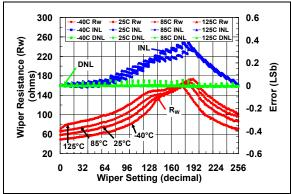
**FIGURE 2-46:** 100 kΩ Rheo Mode –  $R_W$  (Ω), INL (LSb), DNL (LSb) vs. Wiper Setting and Ambient Temperature ( $V_{DD}$  = 3.0V).
