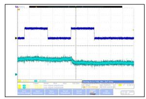
**FIGURE 2-27:** 10 kΩ – Low-Voltage Decrement Wiper Settling Time ( $V_{DD} = 2.7V$ ) (1 μs/Div).
