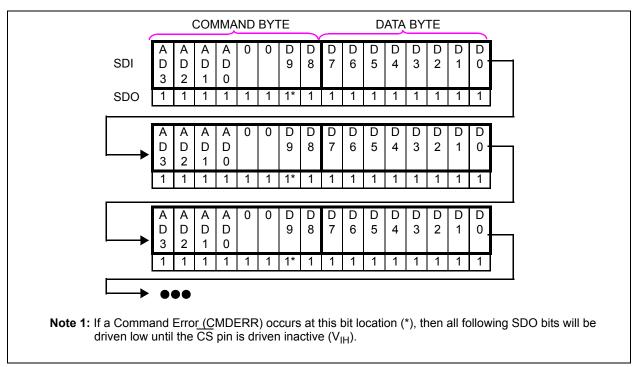
FIGURE 7-3: Continuous Write Sequence.
