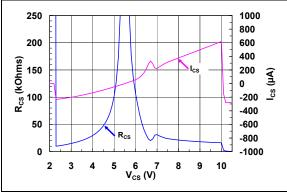
**FIGURE 2-3:**  $\overline{\text{CS}}$  Pull-up/Pull-down Resistance ( $R_{\overline{\text{CS}}}$ ) and Current ( $I_{\overline{\text{CS}}}$ ) vs.  $\overline{\text{CS}}$  Input Voltage ( $V_{\overline{\text{CS}}}$ ) ( $V_{DD} = 5.5V$ ).
