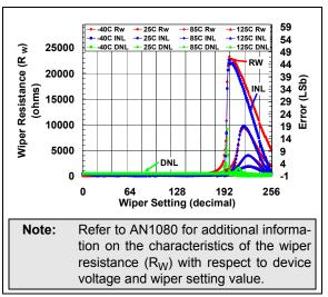
**FIGURE 2-47:** 100  $k\Omega$  Rheo Mode –  $R_W$  ( $\Omega$ ), INL (LSb), DNL (LSb) vs. Wiper Setting and Ambient Temperature ( $V_{DD} = 1.8V$ ).
