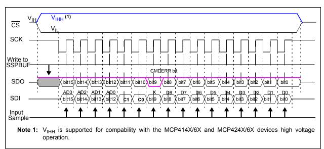
FIGURE 6-3: 16-Bit Commands (Write, Read) - SPI Waveform (Mode 1,1).
