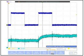
FIGURE 2-40: 50 kΩ – Low-Voltage Increment Wiper Settling Time ( $V_{DD} = 5.5V$ ) (1 μs/Div).
