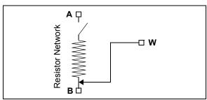
**FIGURE 5-2:** Hardware Shutdown Resistor Network Configuration.
