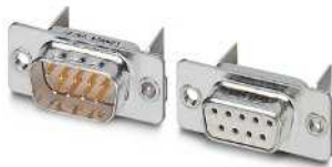
Angled solder pins Fixing: 2.5 mm bore hole and solder metal plate
