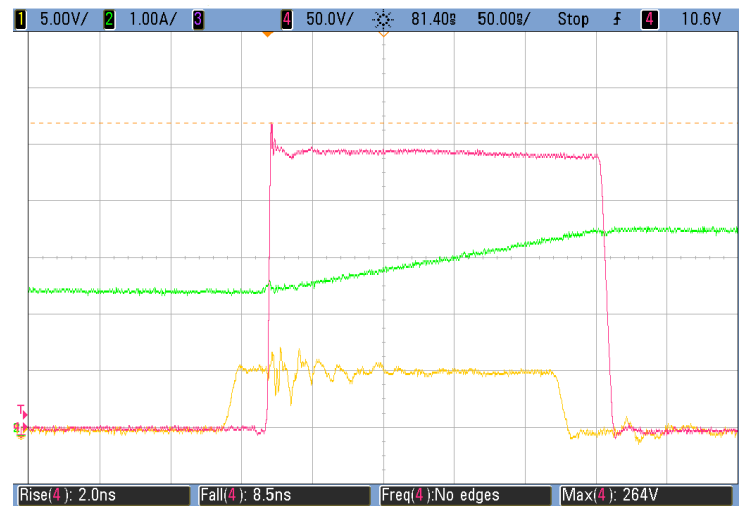
Figure 4: Waveforms for EPC9042, V_{in} = 240\text{ V to }5\text{ V} / 3\text{ A} (100 kHz) Buck converter CH1: PWM Input – CH2: Inductor current – CH4: ( V_{out} ) Switch node voltage
