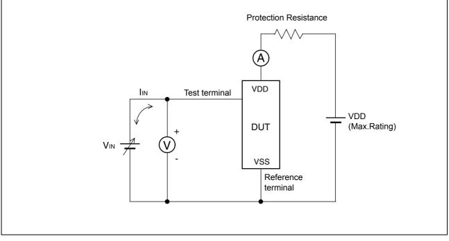
Note : The voltage V<sub>IN</sub> is increased gradually and the current IIN of 300 mA at maximum shall flow. Confirm the latch up does not occur under l<sub>IN</sub> = ± 300 mA.
