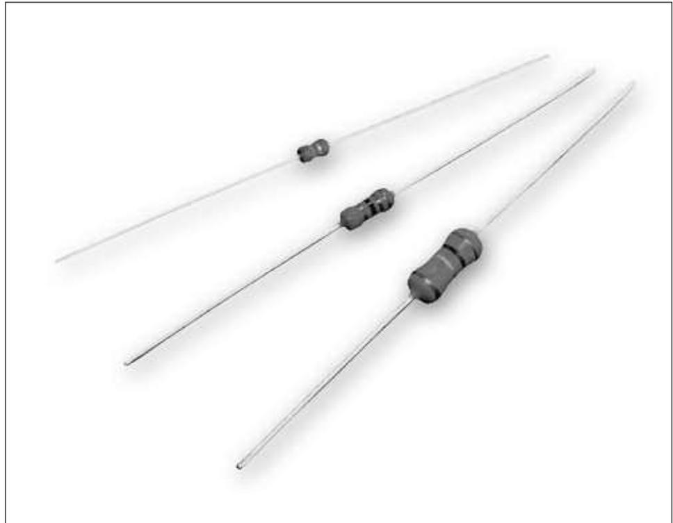
The RR Series is manufactured by depositing a homogeneous film of metal alloy onto a high-grade ceramic body. After a helical groove has been cut in the resistive layer, tinned connecting wires of electrolytic copper are welded to the end-caps. The resistors are coated with a red, non-flammable lacquer, which provides electrical, mechanical and climatic protection. The coating is resistant to all cleaning solvents in accordance with MIL-STD-202, method 215 and IEC 60068-2-45.
