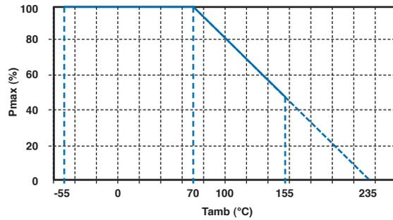
Maximum dissipation (Pmax) in percentage of rated power as a function of ambient temperature (Tamb)
